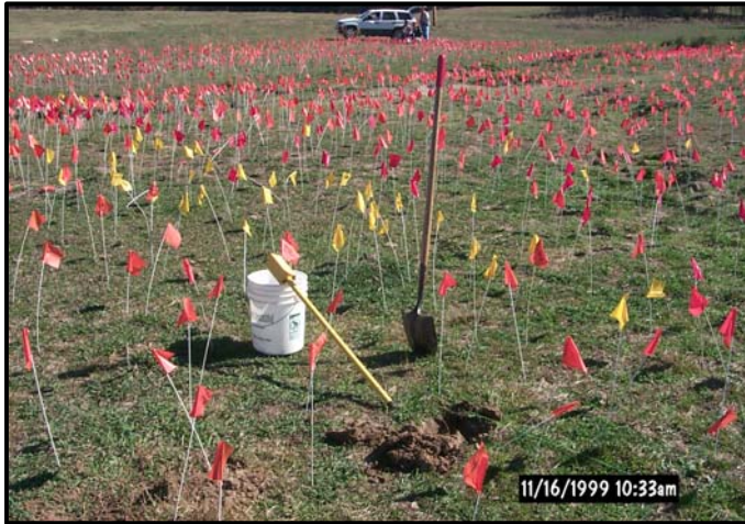
Figure II-26. The Result of Handheld Magnetometer Detection, Known as “Mag and Flag”, is Literally a Sea of Flags, most of which are Non-UXO Metallic Clutter or Geological Features.
