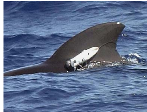
Figure II-17. The Digital Acoustic Recording Tag Developed by Woods Hole Oceanographic Institute (NMFS Permit #981-1578-0).
