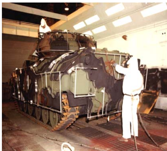
Figure II-24. Typical CARC Painting of a Tracked Vehicle.
