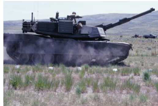
Figure II-19. Tanks and Other Tracked Vehicles Can Damage Plant Cover and Lead to Erosion.
