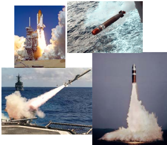
Figure II-4. Rockets that Use Perchlorate-Based Propellants.
